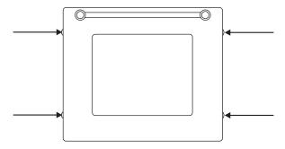
Carefully lift off the outer door panel.
